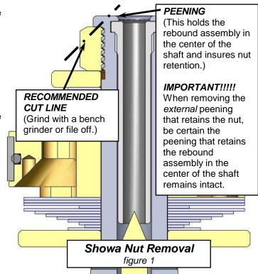
On most KYB's this is not a problem and the peening can be ground off flat, however there are a few models that have a plug in the end and should be treated just like a Showa.
